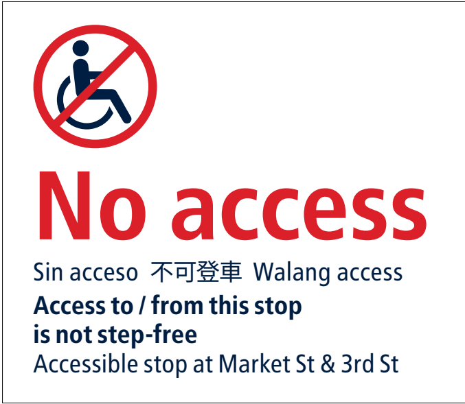
Indicative design Recommended size for alignment with other standard signs proposed at transit stops: 7.5" width x 6.5" height
