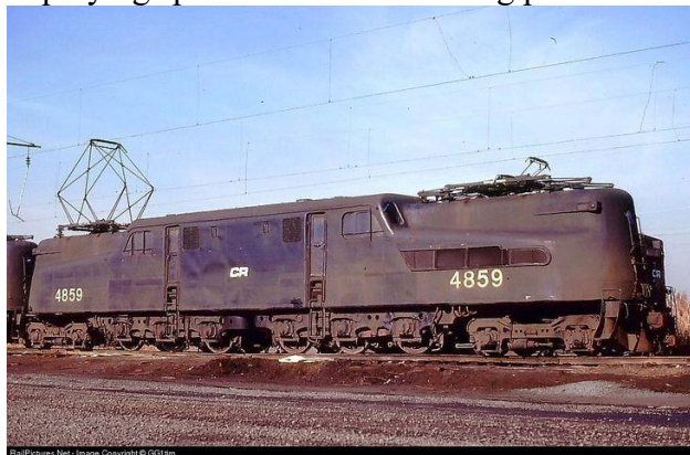
Above is a GG-1 with its pantograph up and in contact with an overhead catenary
