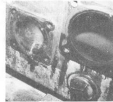
RUPTURED or frozen items on equipment at the Collinwood shop in Cleveland caused by severe low temperatures. (Bernie Cleff photos)
