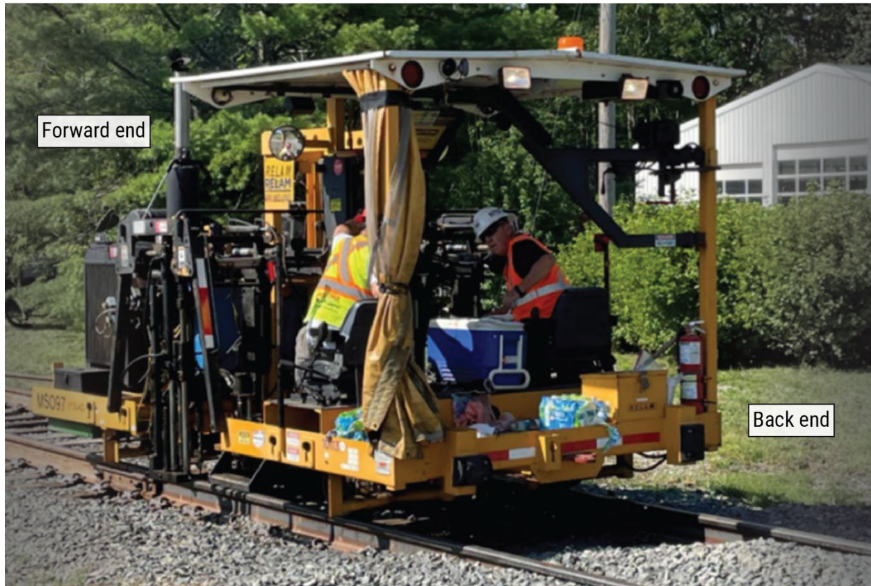
Figure 3. Tie drilling machine MS097 reenactment photograph.
